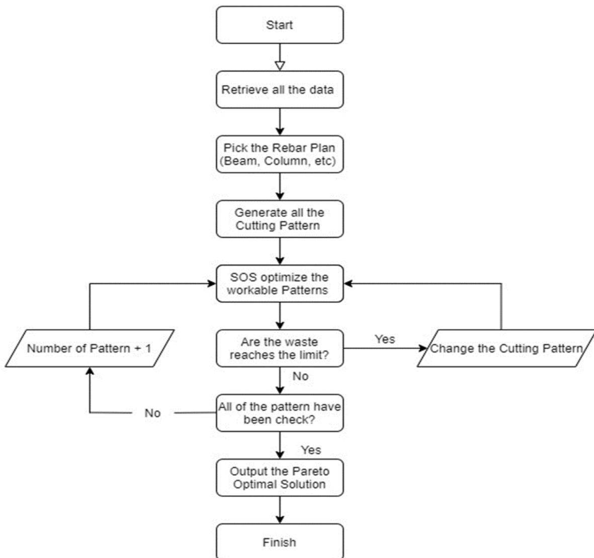
Figure 2. SOS for bi-objective rebar cutting plan flowchart
